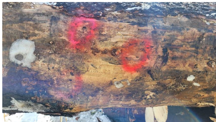
Wood Borer damage – Courtesy of Randy Waterous
