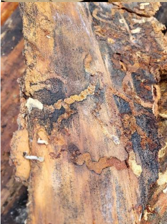
Wood Borer damage – Courtesy of Randy Waterous
