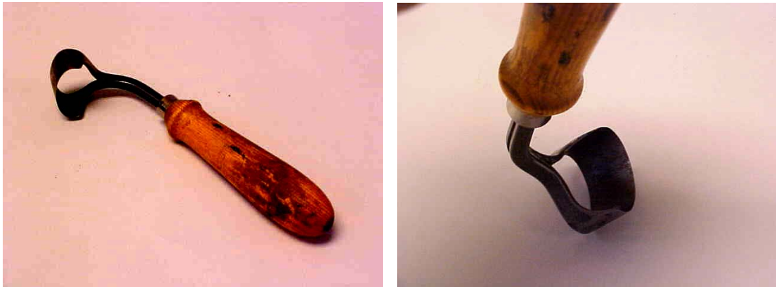
Figure 20: (left) Scorp, a wood-carving tool used for girdling. (right) Close up of blade. Total length of tool is 18 cm.
