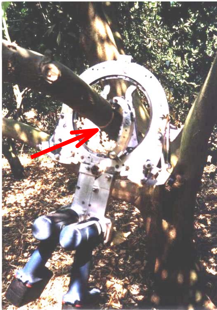
Figure 23: - Mechanical Knife for Girdling . Note fresh girdle cut at arrow.
