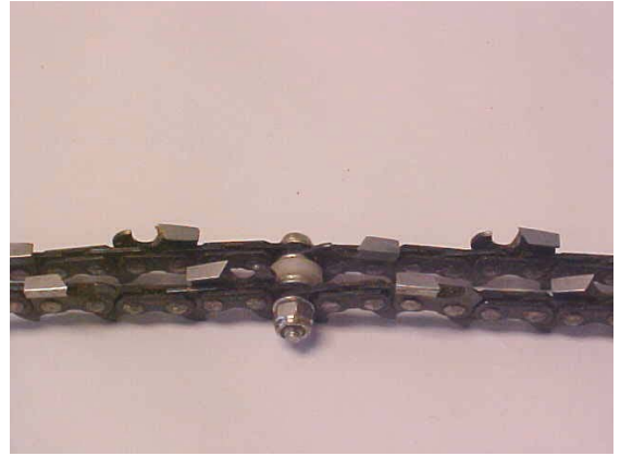
b – Note bi-directional orientation of cutting teeth.
