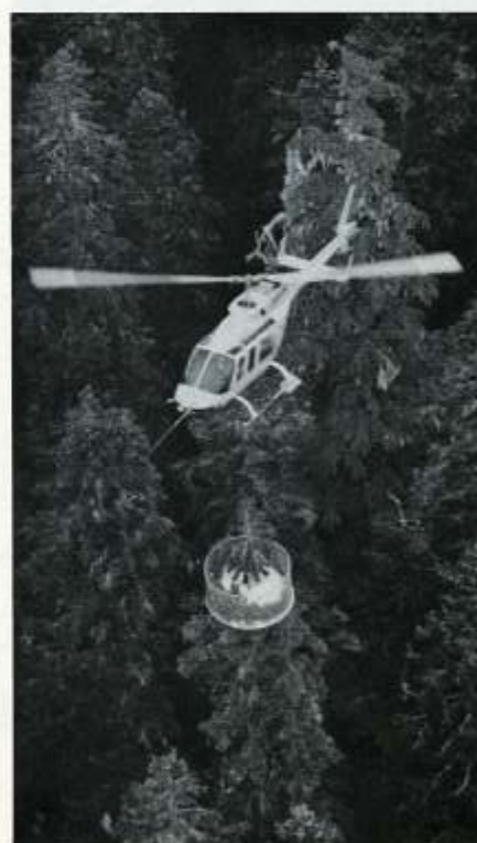
Province-wide cone collection programs use helicopters and cone rakes for high efficiency.
