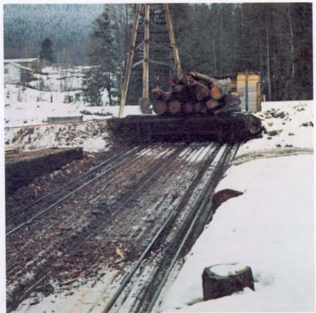
A better way to avoid debris is to ease logs into the water instead of dumping them.
