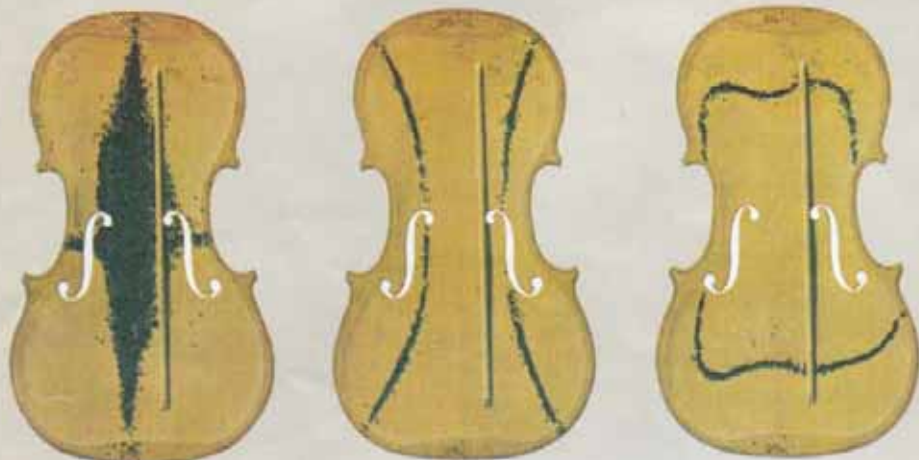
Fine powder sprinkled on a vibrating plate reveals a violin's acoustic patterns. SCIENTIFIC AMERICAN, October 1981.
