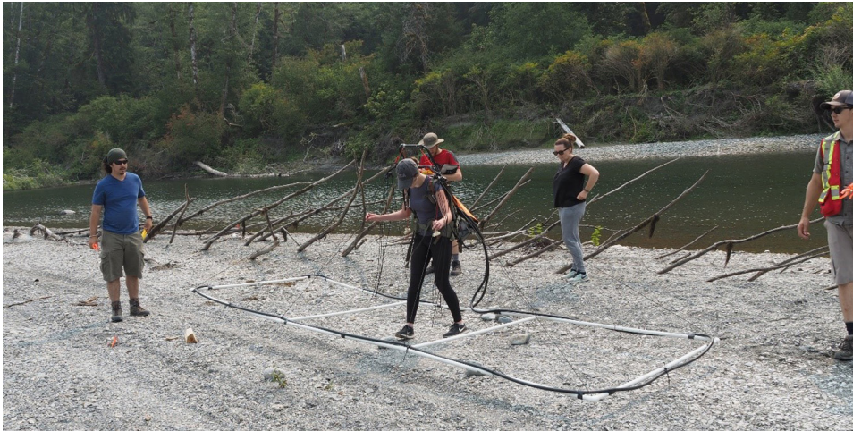
Figure 3. Searching for radio-tagged stones using our large antenna
