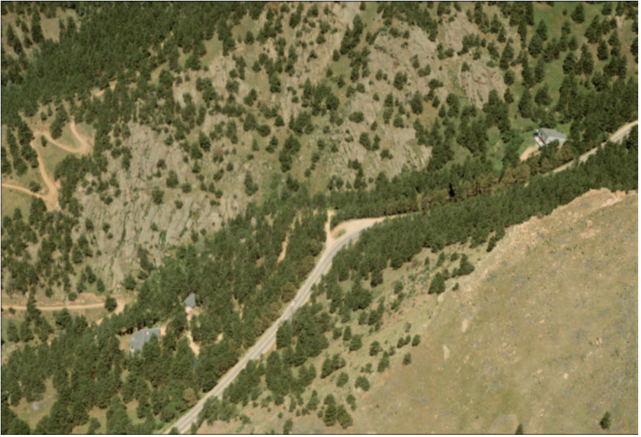
Figure 64. Row of dying ponderosa pines adjacent to a road, probably due to the application of deicing chemicals . Near Boulder, CO.
