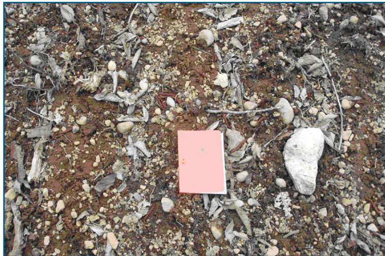
Photograph 4. Bare erodible ground made up 70% of the surface of the ditches in Sections 4 and 5. These sections were also fully connected to the stream.
