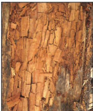
Brown rot – This cube-like type of wood decay is typical of most brown rot.
