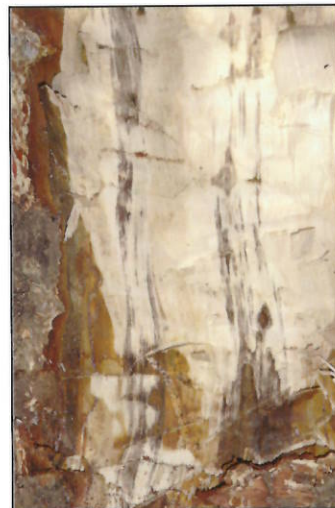
Note the dark streaks in the sapwood caused by blackstain.
