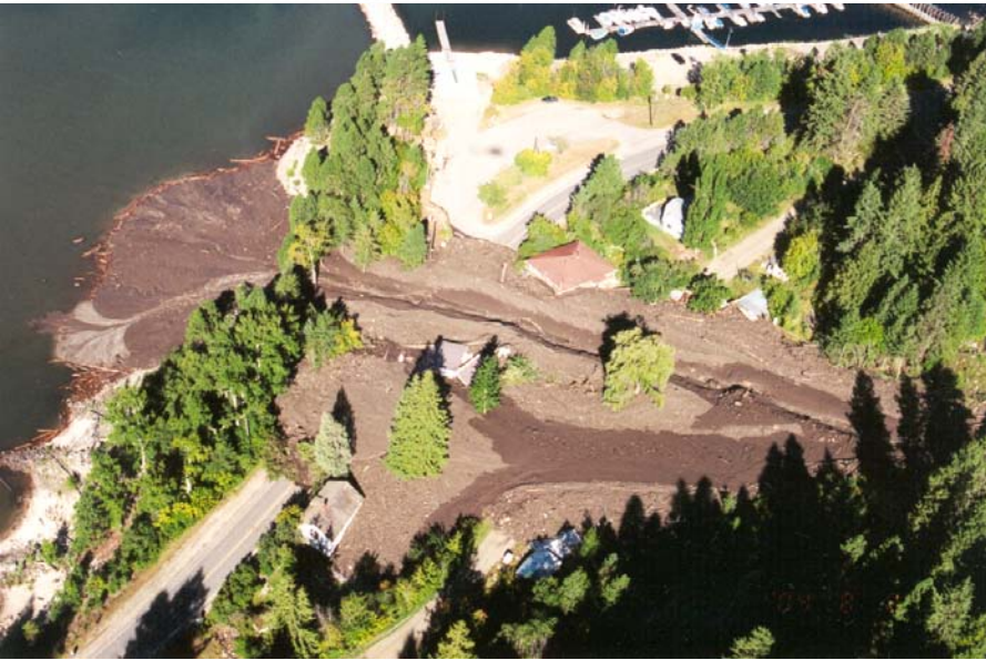
Debris flow deposit on Kuskonook Creek fan. (Photo: P. Jordan). Source: Pike et al. 2010.
