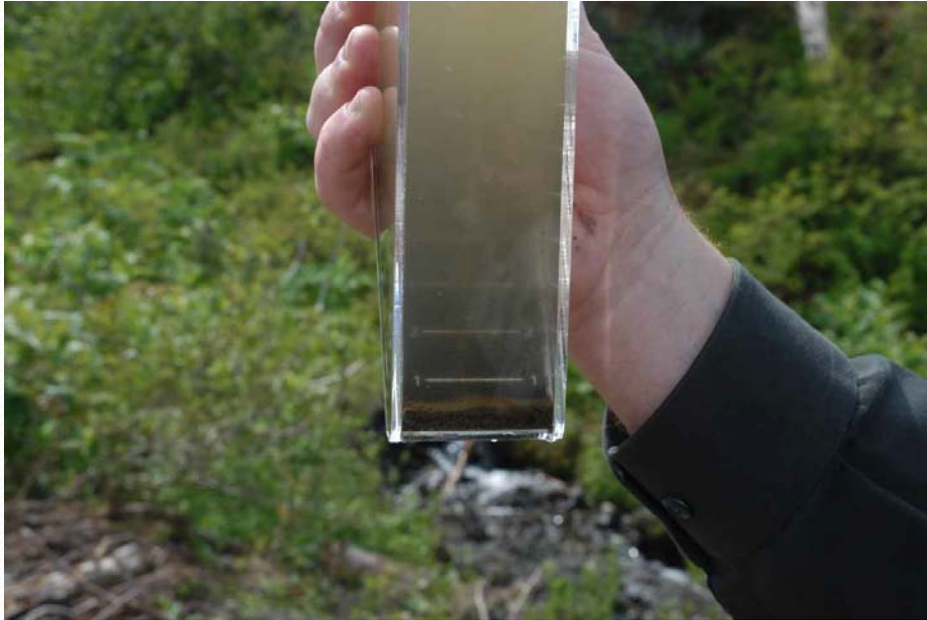
Measuring the turbidity of a water sample. (Photo P. Teti). Source: Pike et al. 2010.
