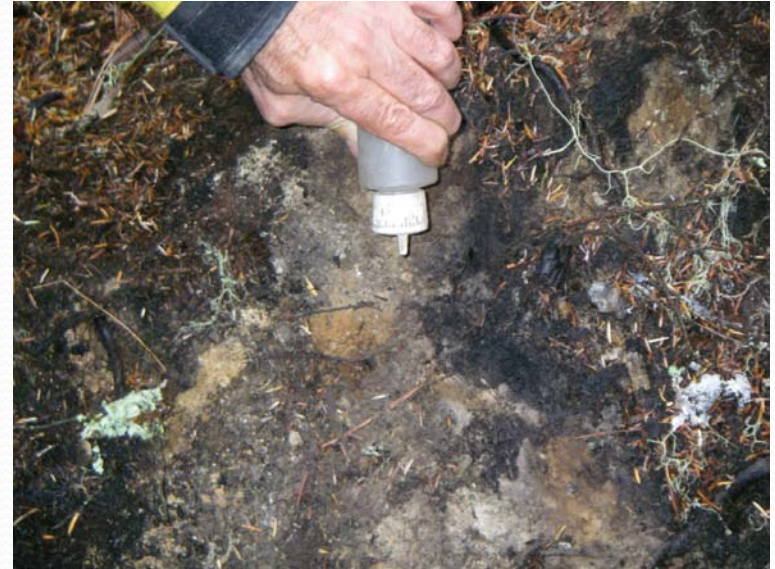
Testing for hydrophobic soil properties. (Photo: R. Pike).
