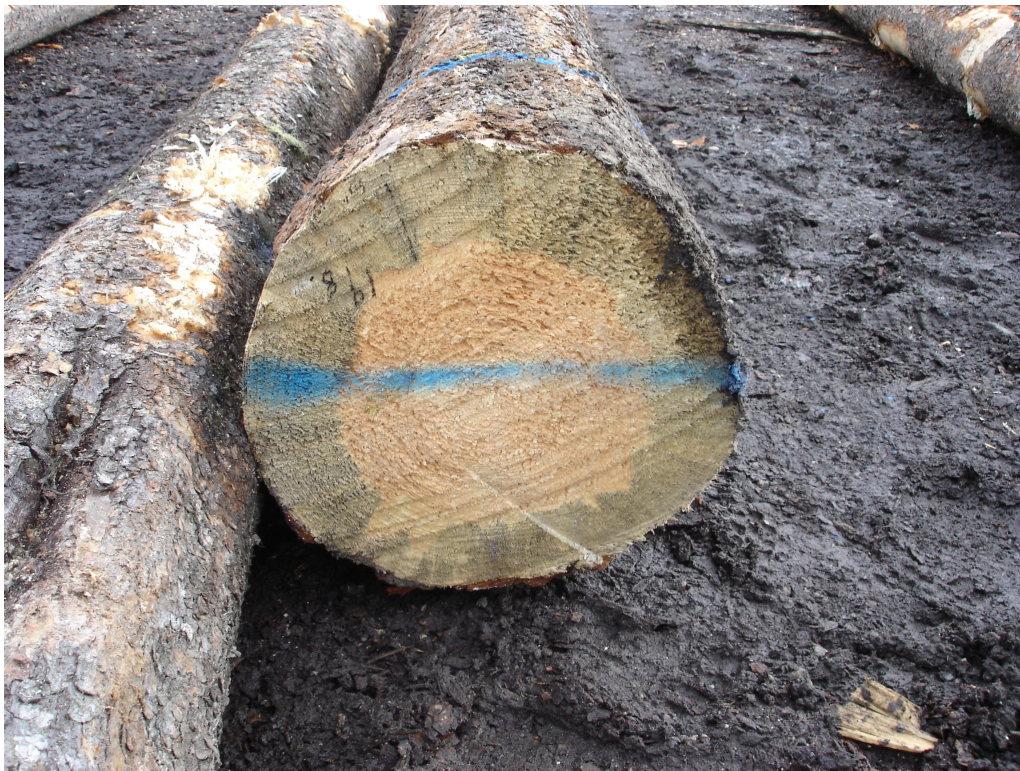
Photo 1 Significant amount of blue stain in a MPB log
