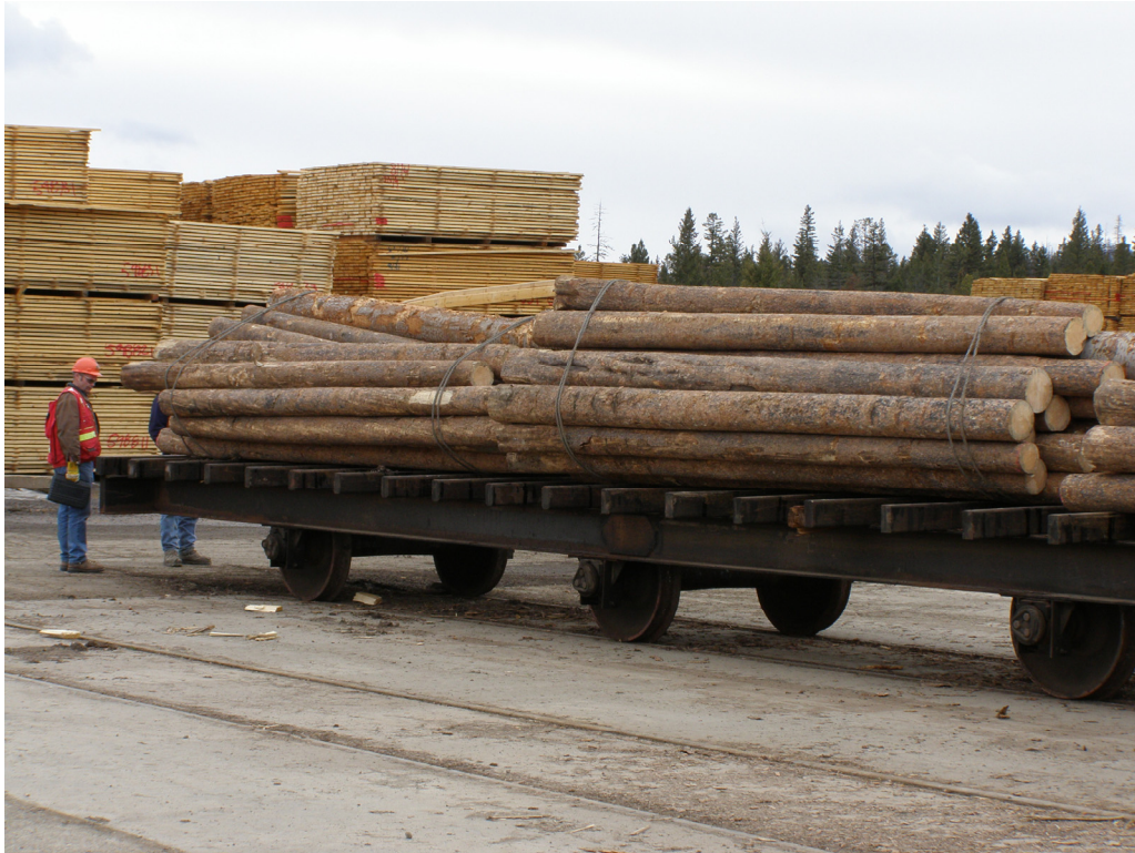
Photo 3 Log charge before entering the kiln
