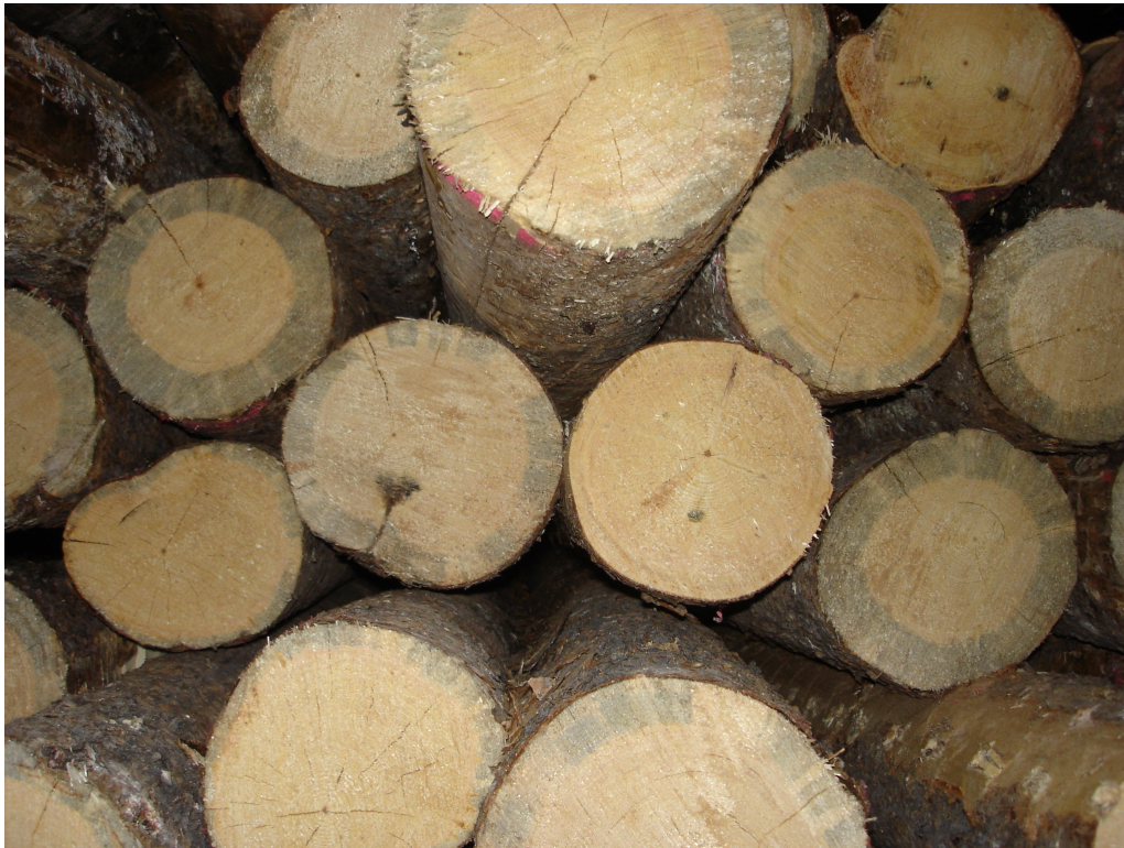
Photo 4 MPB grade 2 and grade 4 logs after re-drying
