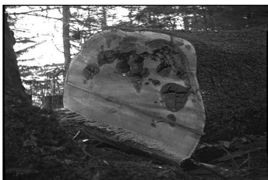
Pocket rot decay caused by N. kauffmanii .
