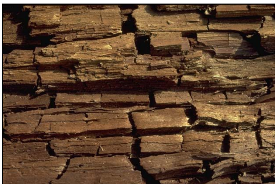
Longitudinal section of brown cubical decay.
