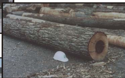
A defective log on a scale site.
