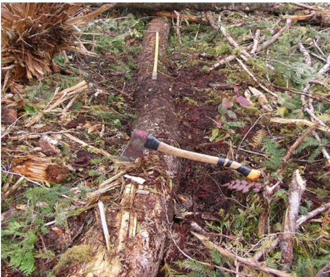
Minor double sweep with straight sections
