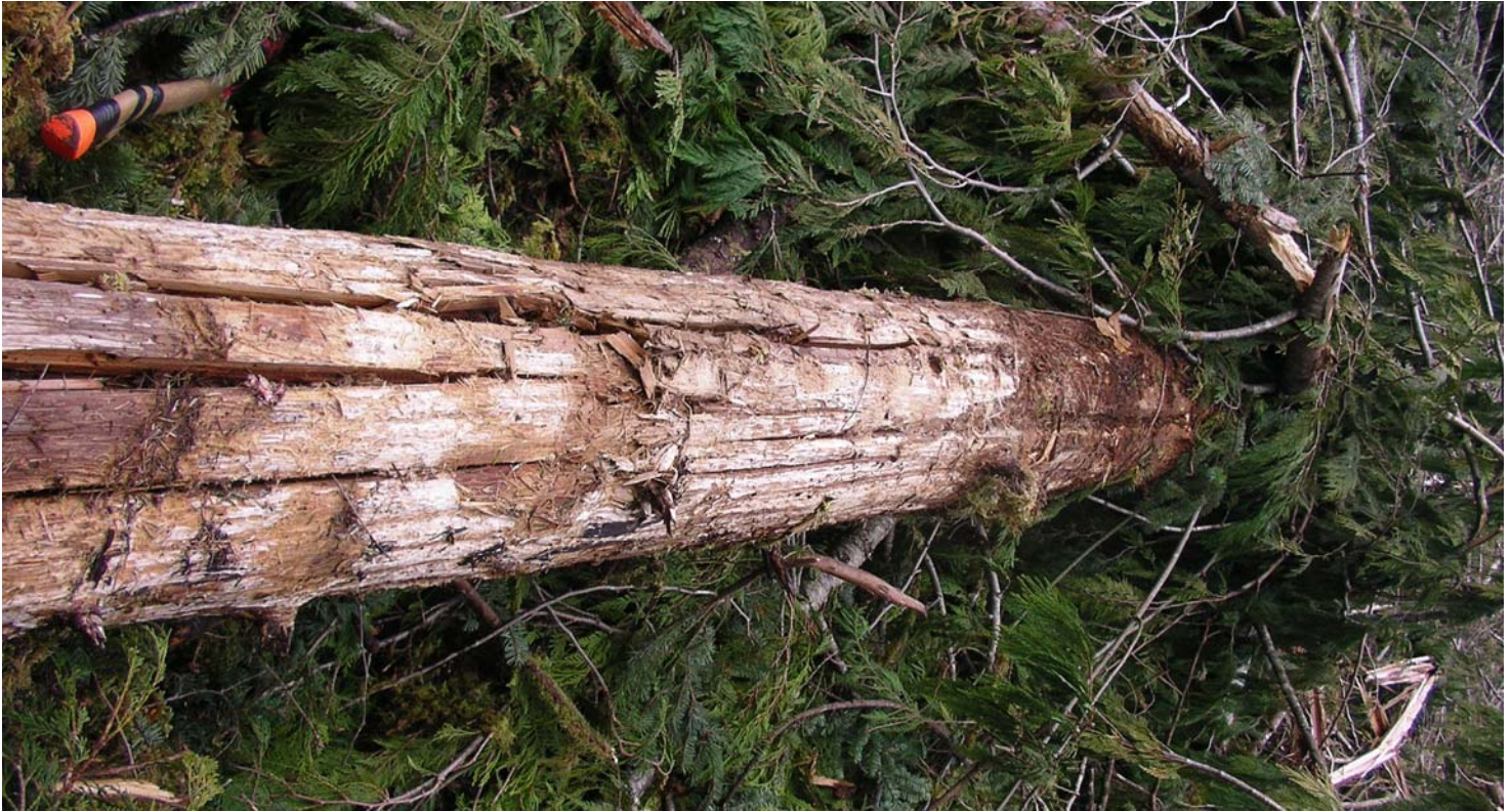
Rotten (hollow) knot on Grey Ghost
