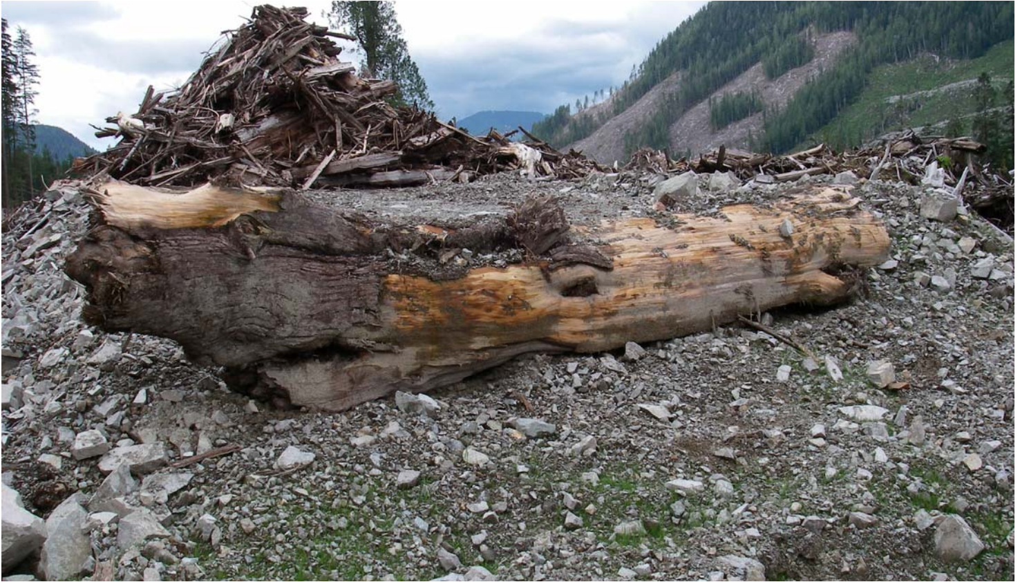
Imbedded rock in Cedar culvert log
