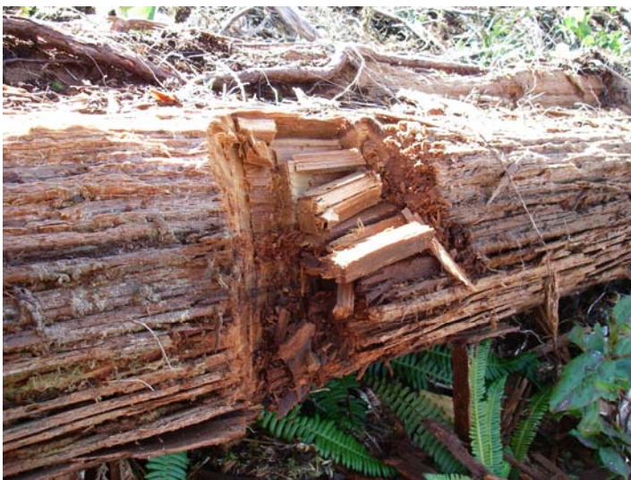
Grain separation deep into log or slab
