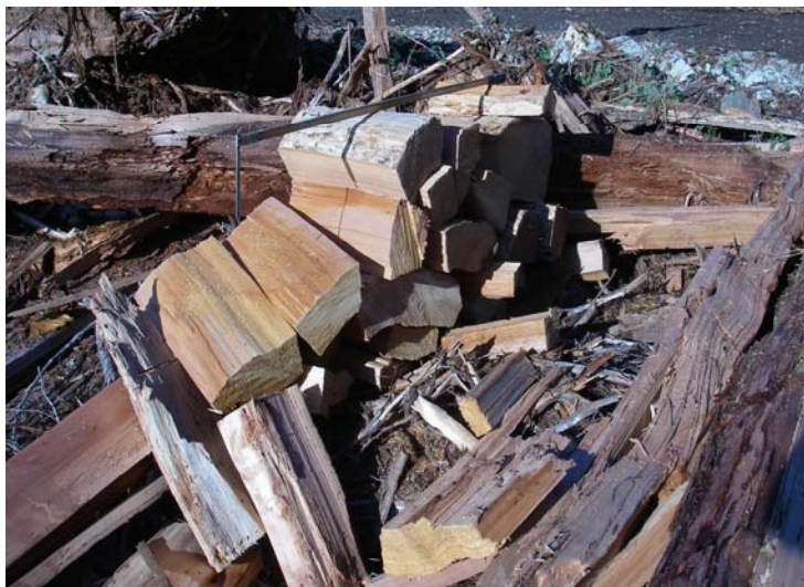
Completed shake bolts and waste material
