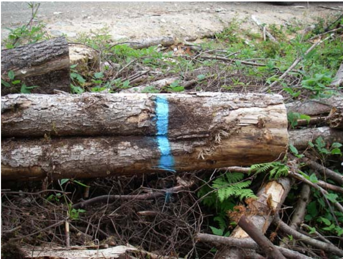
Line shows proper location of buck
