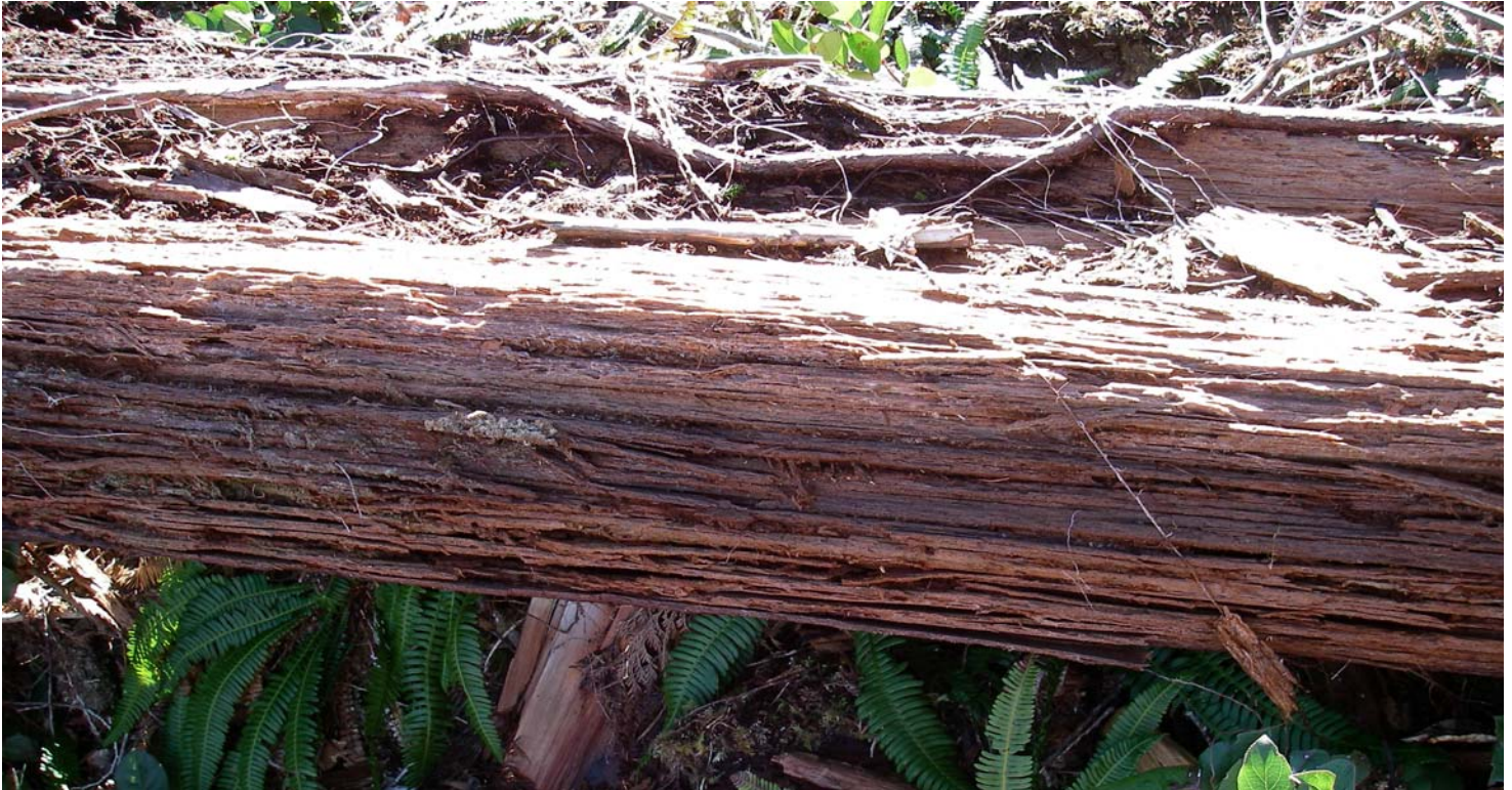
Grain separation deep into log or slab
