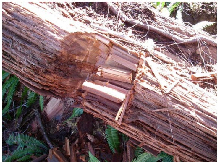
Wood completely unsuitable for lumber
