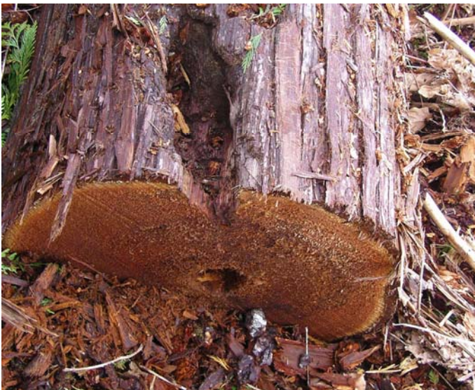
Top end with heart rot and bird holes
