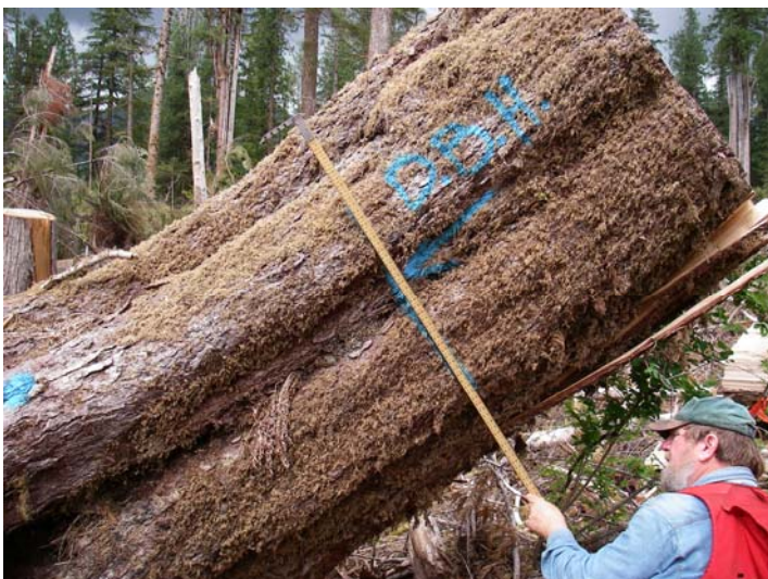
Stump DIB measured at DBH line
