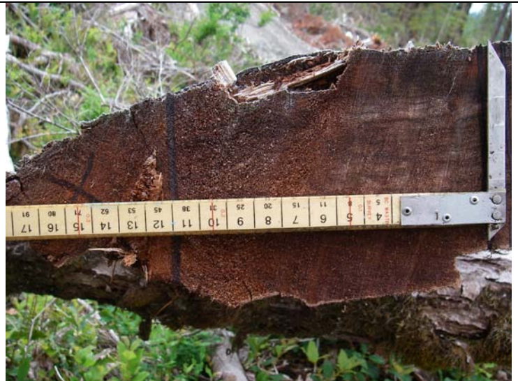
Slab width between TMS edges = 11.5 rads
