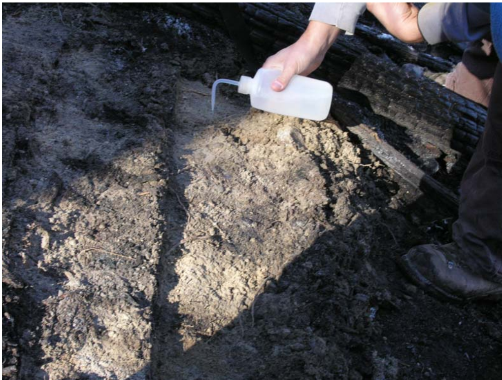
5. Water drop penetration test. Note the drop remaining on the surface, just below the spout.
