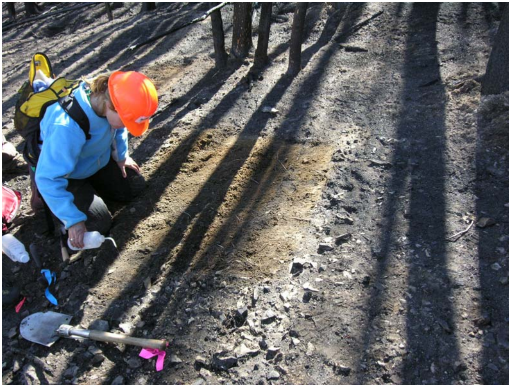
4. Water drop penetration test, at a severely burned plot, Sleetsis fire. Typically, the soil is scraped off to expose surfaces at several depths, and the test is repeated to identify the depths at which repellency exists.
