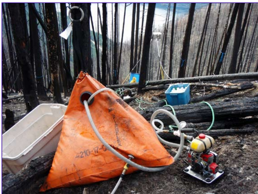
Figure 2. Still-well bladder and small pump supplying water to simulator downslope.
