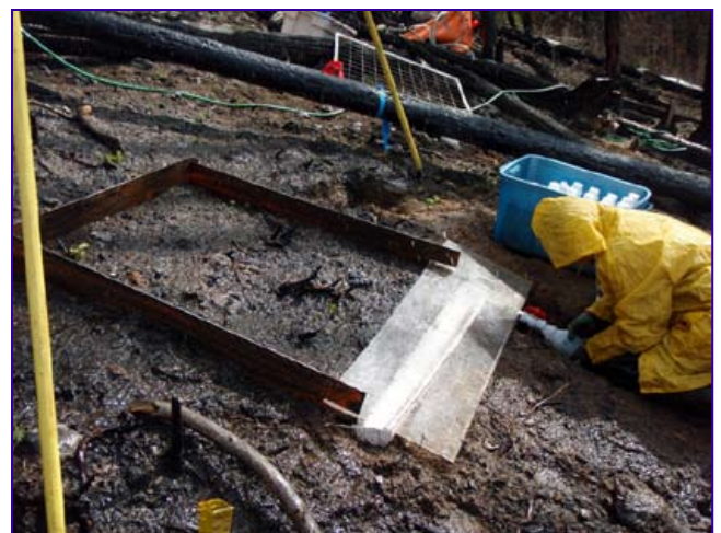
Figure 4. Collecting a sample on a 1-m 2 plot in a high severity burn; note the white collection trough covered by the plexiglas shield.
