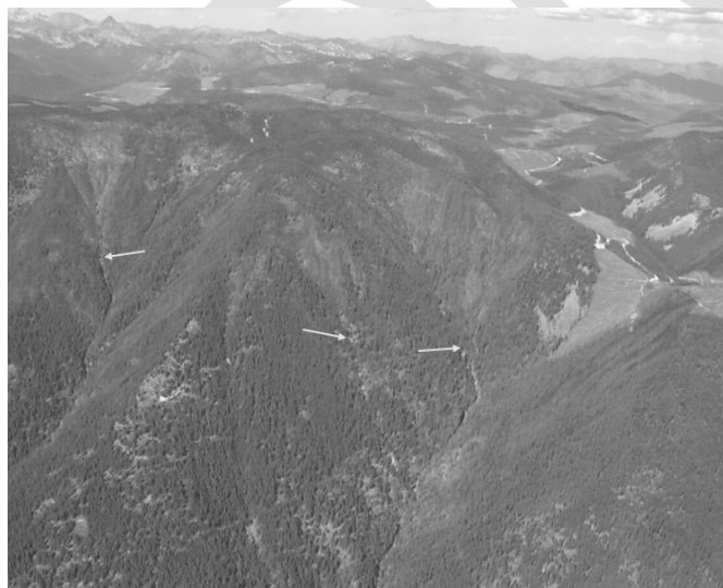
Figure 2. Overview of Kuskonook fire debris flows of August 2004. Debris flow initiation points are shown by arrows.
