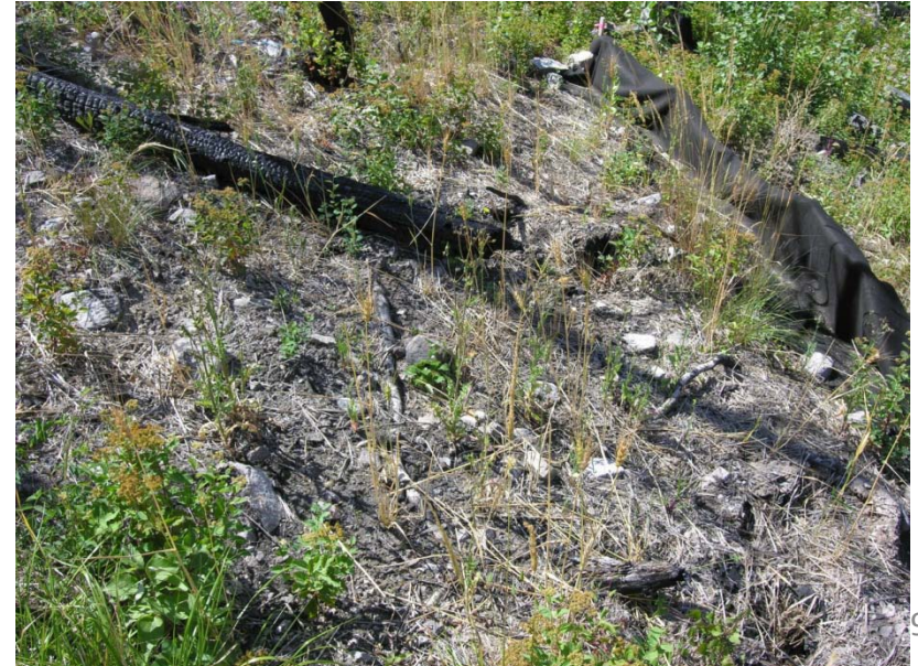
Terrace Mountain: High-severity site, silt fences to test mulch spread by hand
