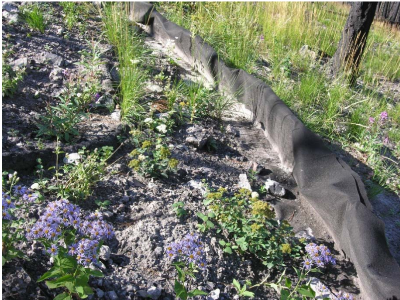
Terrace Mountain: High-severity site, silt fences to test mulch spread by hand
