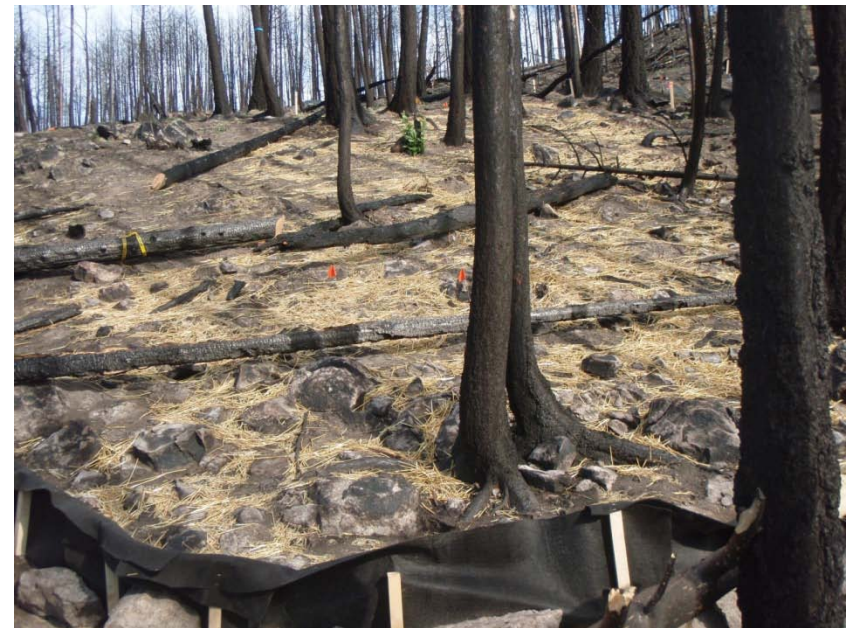
Terrace Mountain: High-severity site, silt fences to test mulch spread by hand
