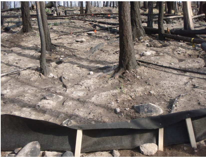
Terrace Mountain: High-severity site, silt fences to test mulch spread by hand
